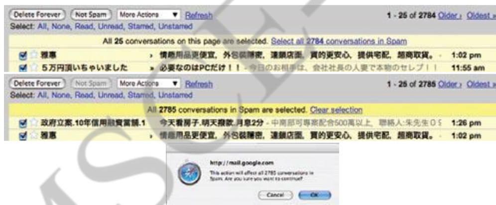
Fig 5.25 Gmail provides a way to select all items across all pages, allowing the user to delete all items in a folder without having to delete all items on each page individually
